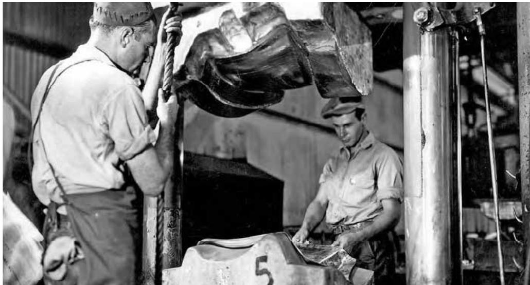
Factory workers used Rohr's "drop hammer" machine to produce thinner and lighter metal for airplanes. The machine had a dramatic effect on the aircraft industry.
